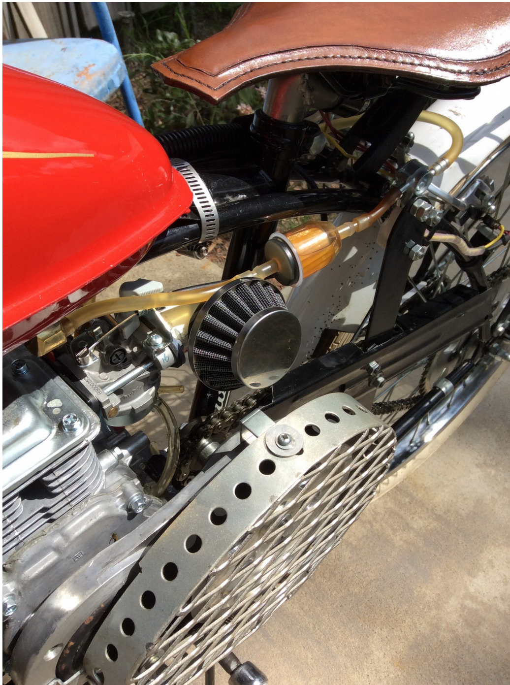
Illustration 1: 35mm Air Filter modification
