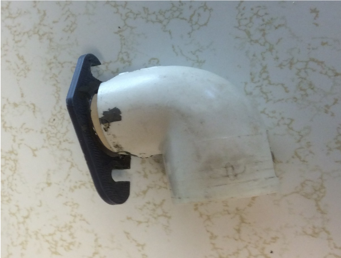
Illustration 2: Compact Intake with 3-D printed flange
