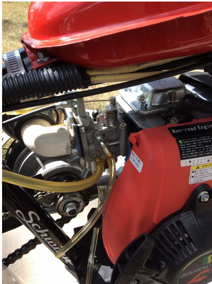
Illustration 4: Right side engine - note clearance with seat tube.
